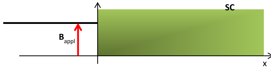
Figure 4. Section of the superconductor, in green. The red arrow represents the magnetic field applied parallel to the surface.
