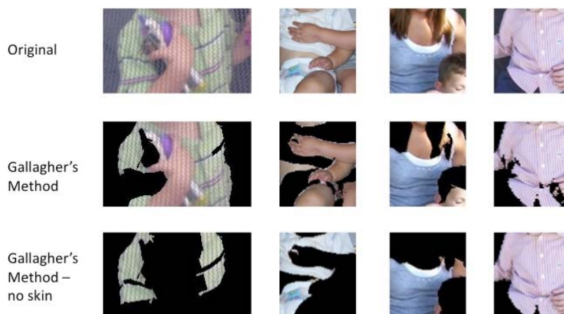
Figure 4.6: Clothing segmented via Gallagher’s method. The seed mask is a rectangular region centered in the image. The final row has been obtained removing skin from the seed mask.
