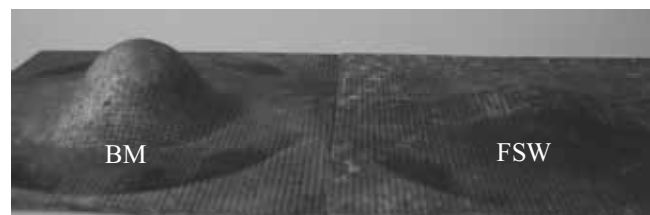
Figure 5. Comparison between BM and FSWed square samples subjected to the hemispherical punch test (350°C; 0.1 mm/s).
