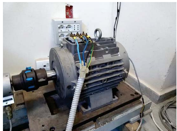
Fig. 5. The three-phase induction motor under test.
