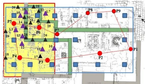
Figure 4. GLS-200 scans position along the traverse path (red circles) in the whole area of the Roman Domus (blue shape). Additional GLS-2000 (violet triangles) and Faro (black triangles) scan positions of the thermal rooms (yellow area with red outline). Internal (green) and external (grey) wooden walkway.
