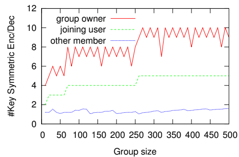
Fig. 9. Number of nodes encrypted/decrypted by using a symmetric schema (y-axis) by the group owner, the other member, and the joining user, for the join of a user to groups of different sizes (x-axis)
