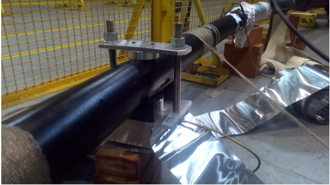
The PEA system for full-size cable. Prysmian Group, Milan.
