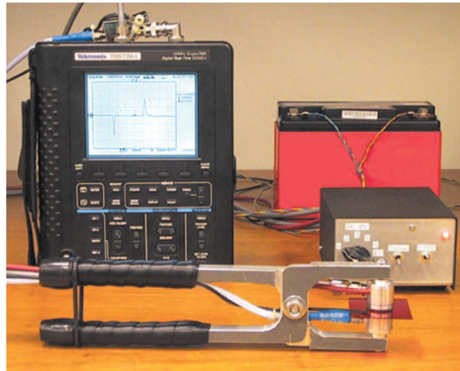
Figure 1.12. Test ground of the Portable PEA [59].
