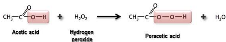
Fig.11 | Reaction of peracetic acid formation.
