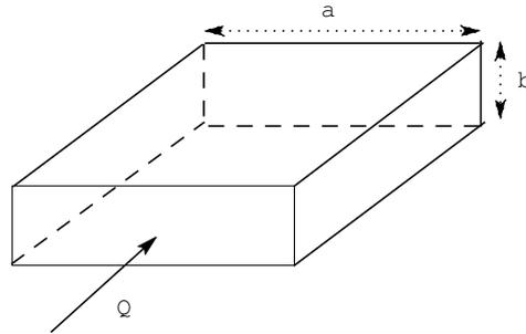
Figure 1. Geometry of the channel being considered with the applied heat flux orthogonal to rectangular section (with size  $a$  and  $b$ ).
