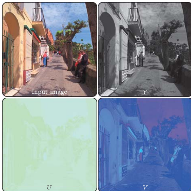
Figure 2: Input image and its YUV channels (U and V emphasized for better display purposes).
