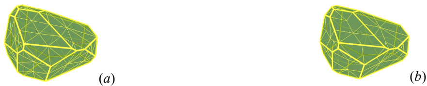
Fig. 3: a ) Surface triangular mesh of a generic grain; b ) Surface mesh of the same grain using the optimized meshing algorithm with triangular and quadrangular elements.
