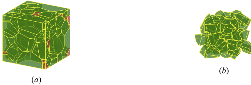
Fig. 1: a ) Periodic morphology as obtained after the cutting process. The grains having a volume less than 10% of the mean grain volume are highlighted. b ) Periodic morphology obtained considering only the grains whose generating seeds fall within the original domain.
