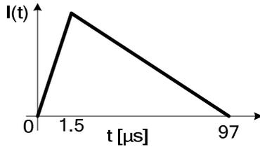
Fig. 7 –Triangular wave, approximating lightning current.
