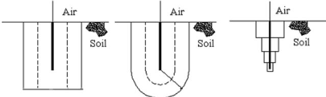
Fig. 1 – Shapes of the supposed ionized zones by Bellaschi, Darveniza and Geri, for a vertical rod. The existence of different conjectures is symptomatic of the difficulty in guessing the shape of the ionized zone.
