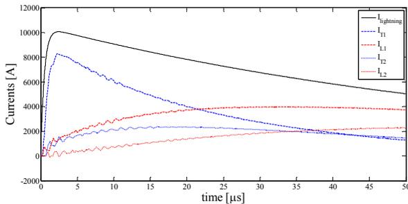
Fig. 11 - Time profiles of currents shown in Fig.10, without considering the ionization phenomenon.
