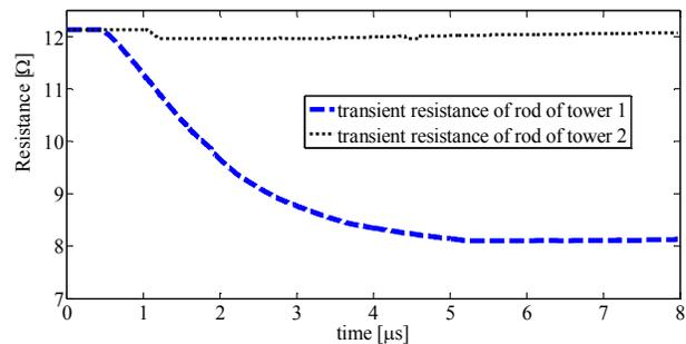
Fig. 14. Time profiles of transient resistance of rods of tower 1 and 2.
