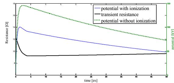
Fig. 9 – Direct stroke on the single rod (no tower simulation) .
