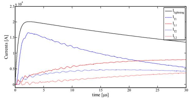
Fig. 13. Time profiles of currents shown in Fig.10, by considering a 20 kA lightning current and neglecting the ionization phenomenon.
