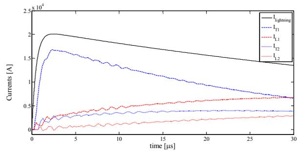
Fig. 14. Time profiles of currents shown in Fig.10, by considering a 20 kA lightning current and implementing the ionization phenomenon.
