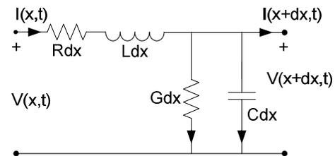
Fig. 3 – Section of the line.
