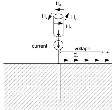
Fig. 2 – Scheme of a vertical rod in a FDTD simulation.
