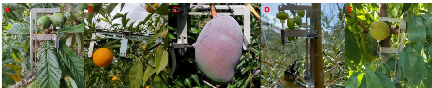
Figure 3. LVDT fruit gauges mounted in loquat (A), orange (B), mango (C), olive (D), and peach (E) fruit.
