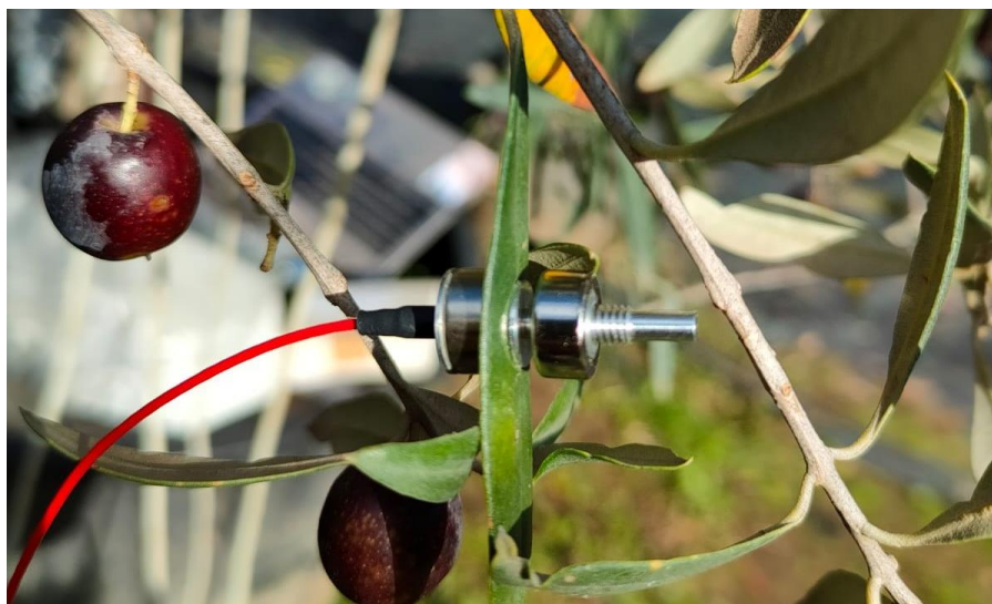
209 Figure 1. LPCP probe mounted in an olive leaf.
