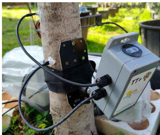
702 Figure 3. TreeTalker® mounted on an olive trunk.
