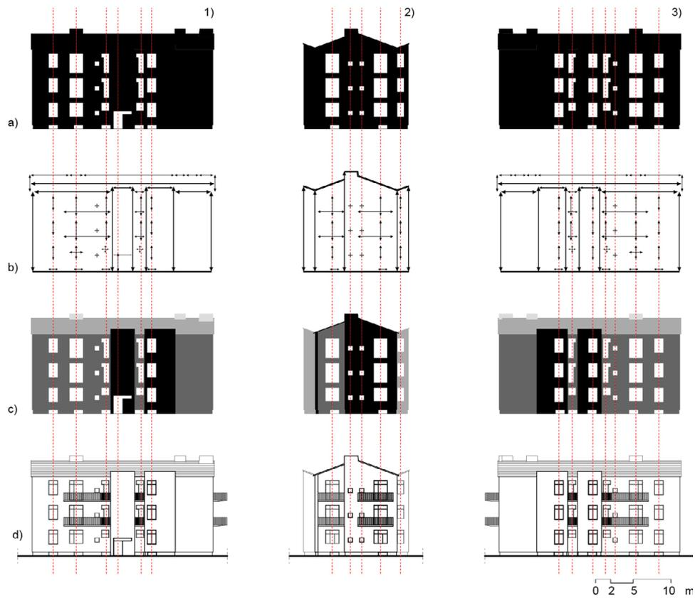
Fig. 6. Vico Magistretti, project for the workers' houses at the Cotonificio Olcese in Cagno (BS), graphic analysis: a) full-empty ratio; b) comparison of horizontal-vertical vectors; c) depth planes; d) two-dimensional graphic model of the building. Elaborations by the author.
