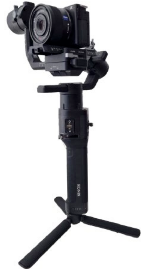
Fig. 14 – Sony ZV-1 Camera mounted on a 3-axis stabilized DJI Ronin-SC.
