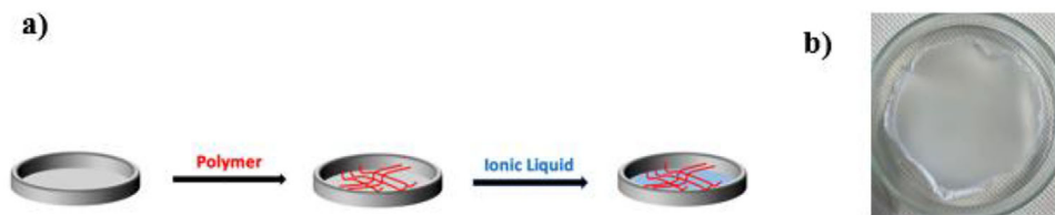
FIGURE 2 | Schematic depiction of (a) membrane preparation and (b) representative picture of an IL-doped PHB membrane.
