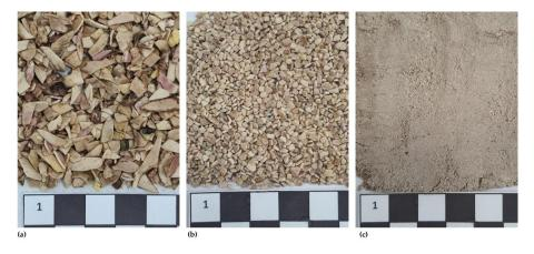
**Figure 2.** Pistachio shell grain sizes: (**a**) Pg shells with dimensions ranging from 2 to 4 mm; (**b**) Pf shells with dimensions of 0.5–2 mm; (**c**) Ps shells with dimensions <0.5 mm. Figures report the metric reference to 1 cm.
