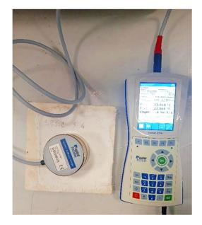
Figure 7. ISOMET 2114 thermofluximeter in operation.
