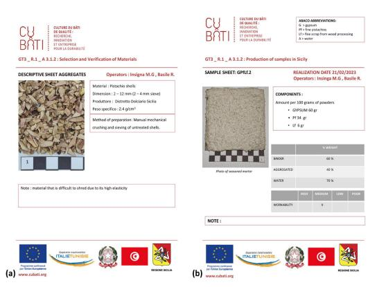
Figure 1. Record cards: (a) aggregates; (b) mix designs.
