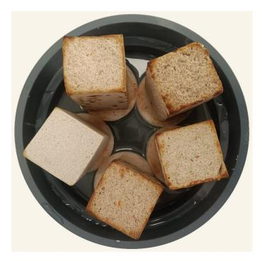
Figure 6. Water absorption test by capillarity.
