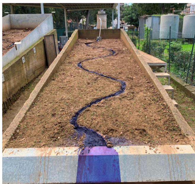
Fig. 2. – View of the wetted portion of the rill channel highlighted by the Methylene blue solution for CS.
