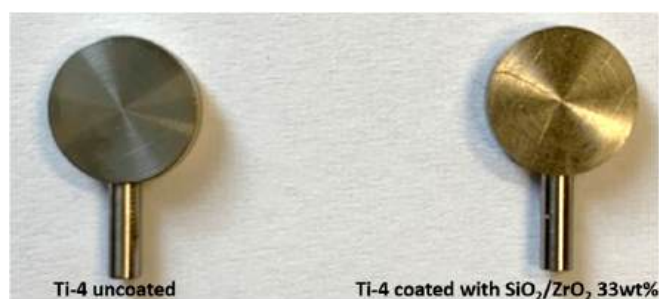
Figure 2. Representative images of the commercial Grade 4 titanium (Ti-4) disks: Untreated disk (left) and disk coated with SiO 2 /ZrO 2 (33 wt.%) (right).
