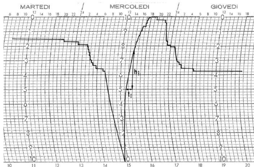
Figure 2.4.1 - Hyetograph divided into m parts, each with constant rainfall intensity.
