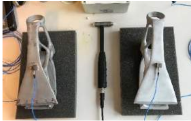
Figure 1 additive and subtractive mechanical components under impact loading
