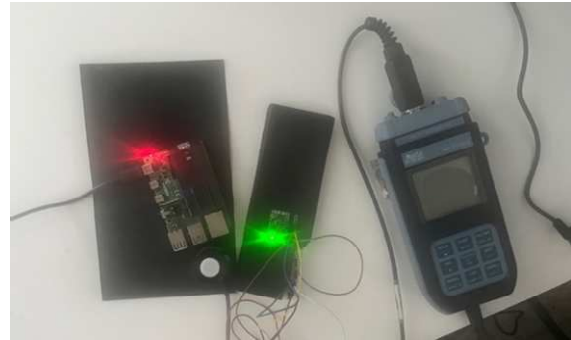
Fig. 3. The instrumentation used during the first measurement campaign: Arduino, Raspberry, and Delta Ohm luxmeter.
