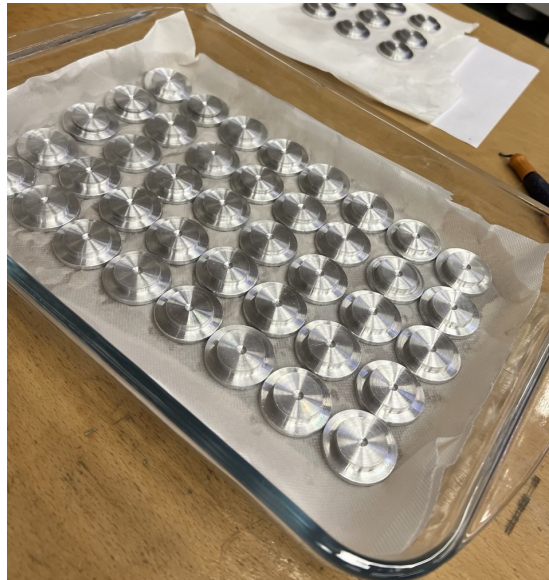
Figure 5.5 Batch in a tray of machined and cleaned high-purity (99.999%) aluminum anodes produced for the refurbishment and future test activities of the Penning source. In conditions of low Ar pressure ( \sim 7 \times 10^{-5} mbar), high current ( 1 \div 2 A), the intensity of recombination lines of Al v near 108 Å produced by the source will be maximized.
