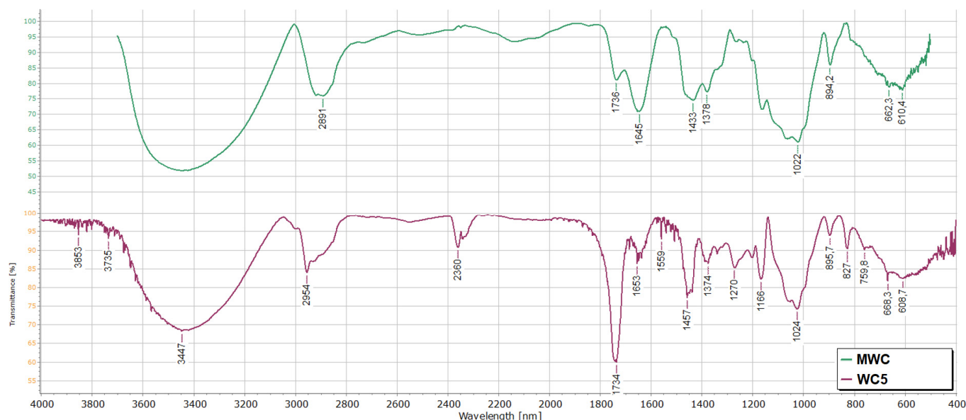
Figure 2. FTIR spectra of cellulose derived from CPWs after mercerization (top curve in green) and WC5; the material at a high degree of functionalization (bottom curve in purple).
