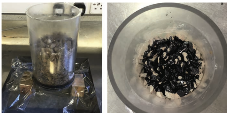
FIGURE 1. Flowability test apparatus and specimen set up.
