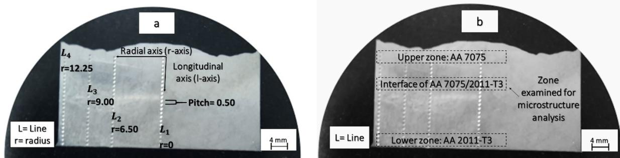
Figure 2. Schematic diagram for (a) Vickers hardness test, and (b) microstructure analysis
