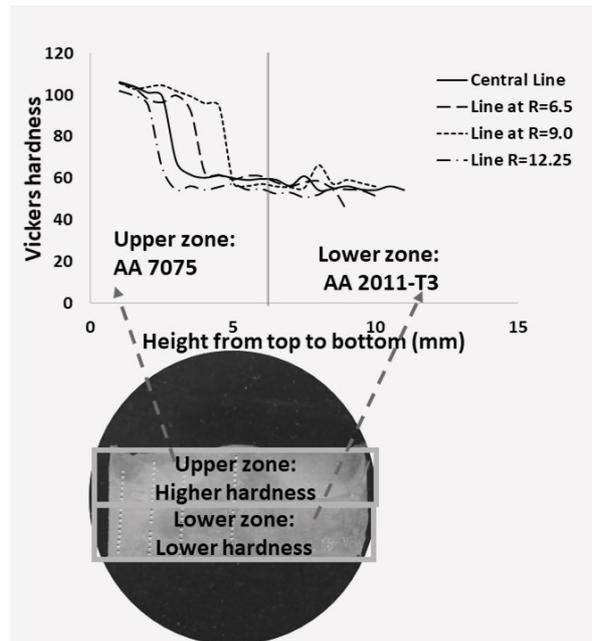
Figure 3. Hardness profile of AA 7075/2011-T3 billet
