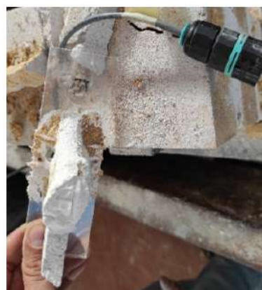
Figure 17. Sensor fully embedded after the test.
