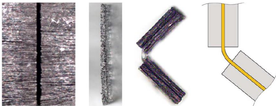
Figure 7.3. Details on the production sequence of flexible joints through Smart Composite Microstructure technique [62]
