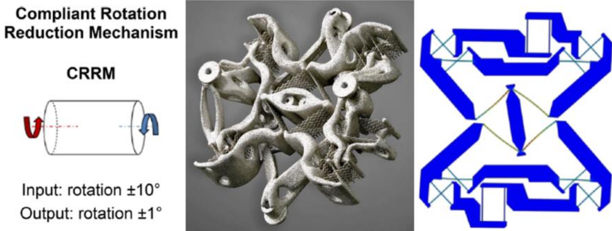
Figure 2.3. Compliant rotation reduction mechanism, concept, prototype and FEA
