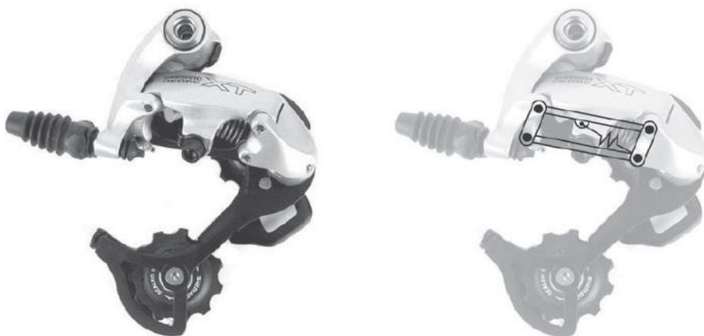
Figure 2.13. Bicycle derailleur and a representation of his rigid body mechanism mechanism, it has to be chosen the rigid components to be replaced with flexible ones, in this case represented by one compliant fixed-fixed beam.
