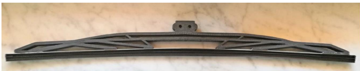
Figure 6.8. FDM prototype of compliant monolithic frame realized in Nylforce CF[54]
