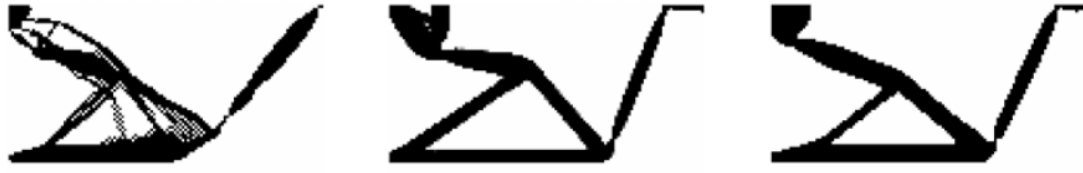
Figure 3.10. Optimized CM inverter (left) and two different filters applied: density filter with linearly decaying weighting (center) and bi-lateral density filter (right) [37]
