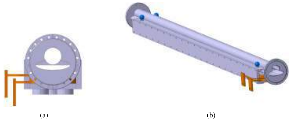
Fig. 6.21 Mechanical drawing of the Lambertson septum for booster injection in a cross-section side view (a) and isometric view (b)
