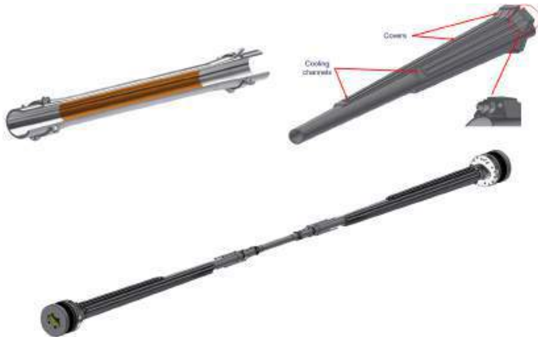
Fig. 1.29 Top Left: Central chamber including cooling inlets and outlets for the paraffin cooling circuit housed in a double layer and its internal gold coating layer; Top Right: ellipto-conical vacuum chamber with asymmetric cooling channels; Bottom: assembly of the IR chambers
