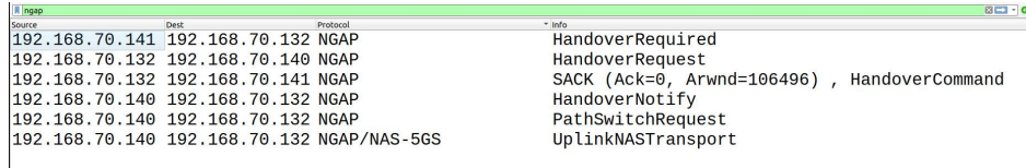
Figure 4: Wireshark message captured during handover procedure.
