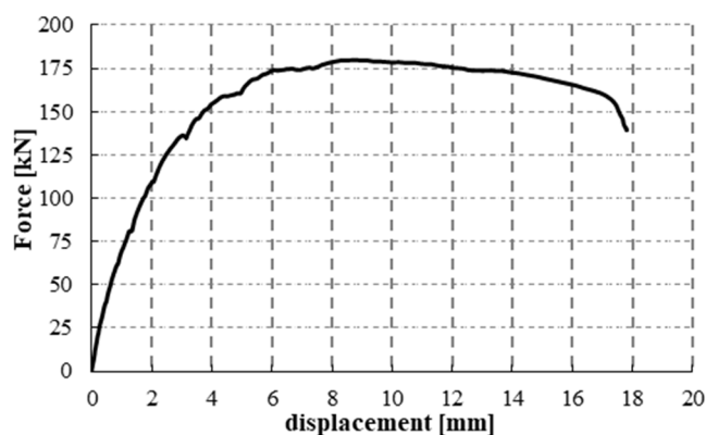
Figure 2 Force-displacement response of the reference experimental test
