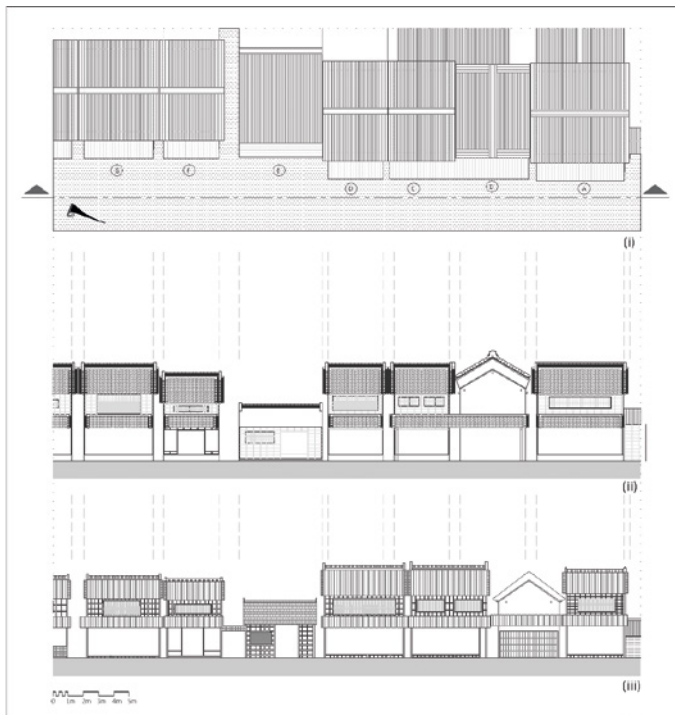
Figure 7 Comparison of the building footprints with street elevation: (i) site plan showing building footprints; (ii) proposed facade composition based on the digital interpretation; and (iii) digital reproduction of the facades by Ito 2003
