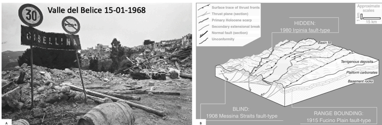
Fig. 1 – A) Picture of the epicentre of the 1968, Mw 6.4 Valle del Belice earthquake whose “elusive” seismogenic source is still debated; B) Types of “elusive” faults from Valensise, G. & Pantosti, D., (2001). Journal of Seismology . https://doi.org/10.1023/A:1011463223440
