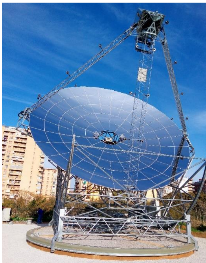
Figure 11. The dish-Stirling reference system installed at the university campus in Palermo (Italy)
