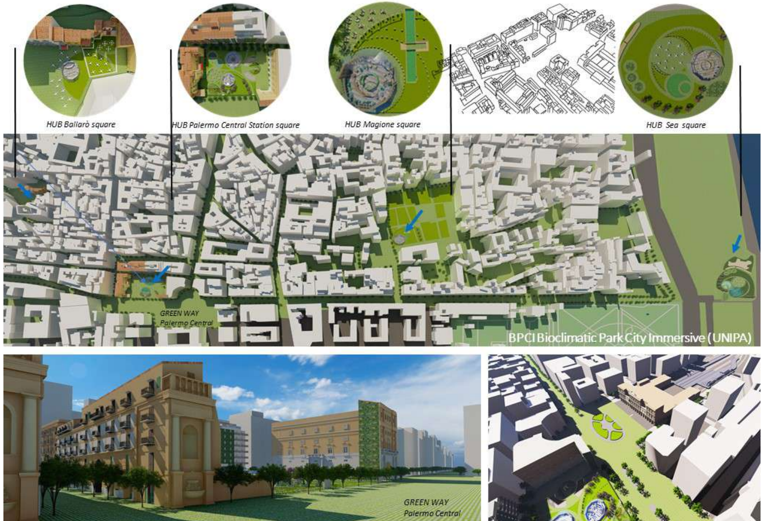
Fig. 7 - Masterplan of the Green Way (from Corso Tukory to piazza Abramo Lincoln and sea) indicating the strategies and intervention measures, and specific actions of retrofitting of the public spaces subject to modelling and simulation
