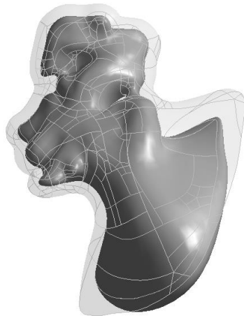
Figure 34 This figure shows the STEP model of the left atrial appendage in the internal part after post processing in Rhinoceros.
