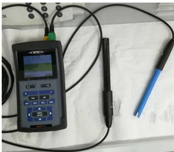
**Figura 3. 13. Multimetro WTW Multi 3420**
