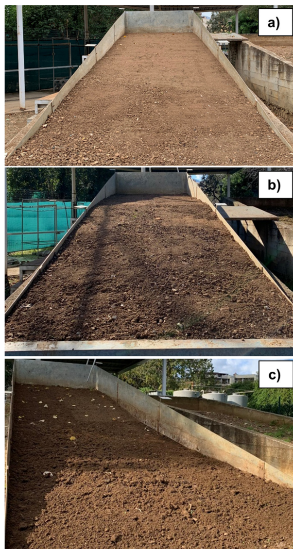
Figure 1. View of the experimental plot with uniform (a), convex (b), and concave (c) profiles.
