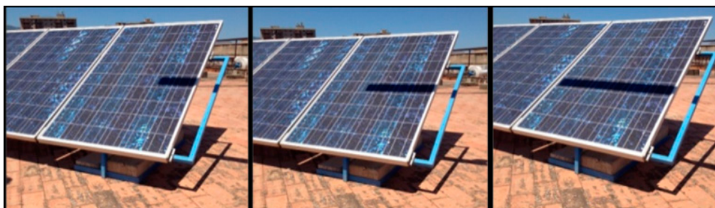
Figure 8. Shaded panel case 1, 2 and 3. In case 1 shadow can vary from 225 to 450 cm 2 ; which corresponds to one interruption of a line of cells; in case 2 shadow varies from 450 to 900 cm 2 , which corresponds to two interruption of lines; case 3 corresponds to the interruption of the panel.
