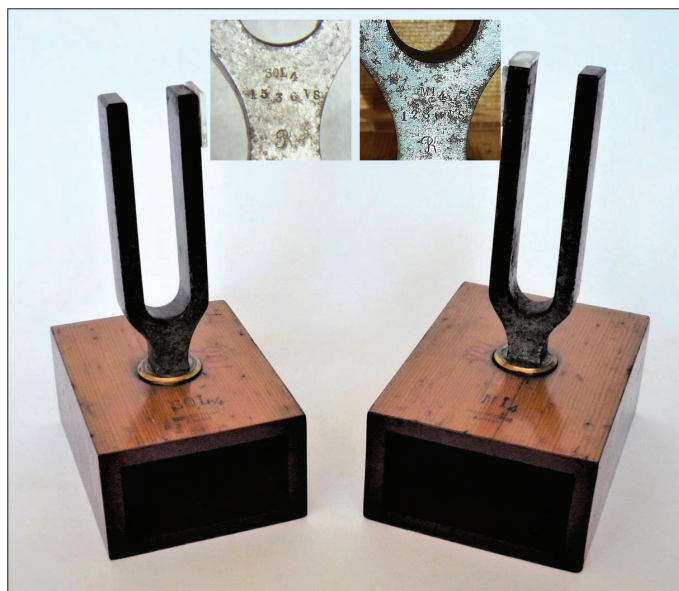
Fig. 1. Photo of the tuning forks on wooden ( Picea abies ) resonance box produced by Koenig and bought by Blaserna in 1868. 3,4 The insets show the resonance frequency and the manufacturer's monogram, engraved on the tuning forks. Historical Collection of the Physics Instruments of the University of Palermo, Italy.
