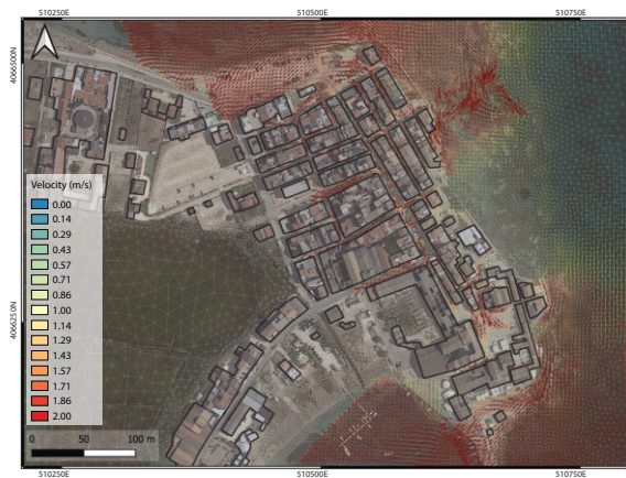
Figure 8. Example of the vectorial velocity field. Coordinate reference system: EPSG 32632.
