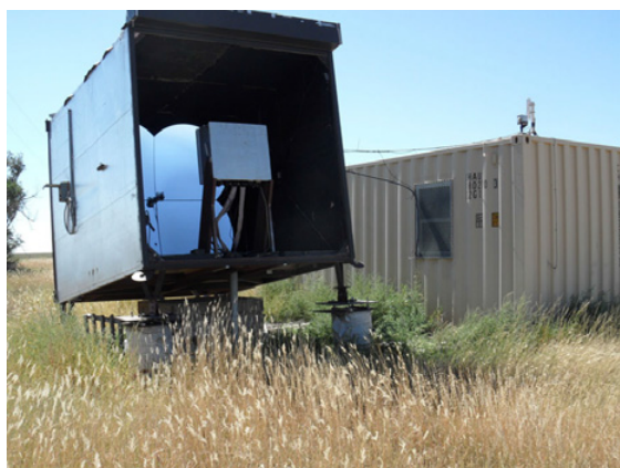
Figure 7. The AMT: on the left, the 4-segment spherical mirror and the camera housed within the waterproof shelter. The office container next to the telescope hosts all the computers.
