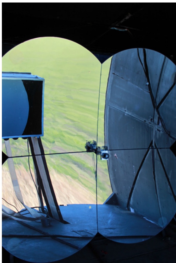
Figure 6. The 4-segment spherical mirror and the LED facility. The camera, equipped with the UV filter, is reflected in the mirror.
