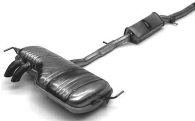
Figure 1.4 Commercial exhaust system made of titanium (Source: [3]).
