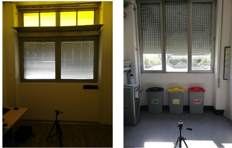
Figure 22 – (a) Inside view of second floor room (SW-LSC) – (b) Inside view of first floor room (traditional window)
