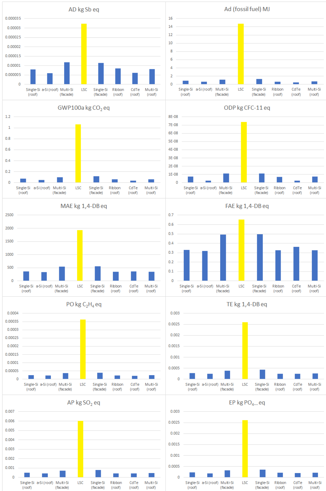
Figure 54 - Environmental impacts comparison between different PV modules (1 kWh)
