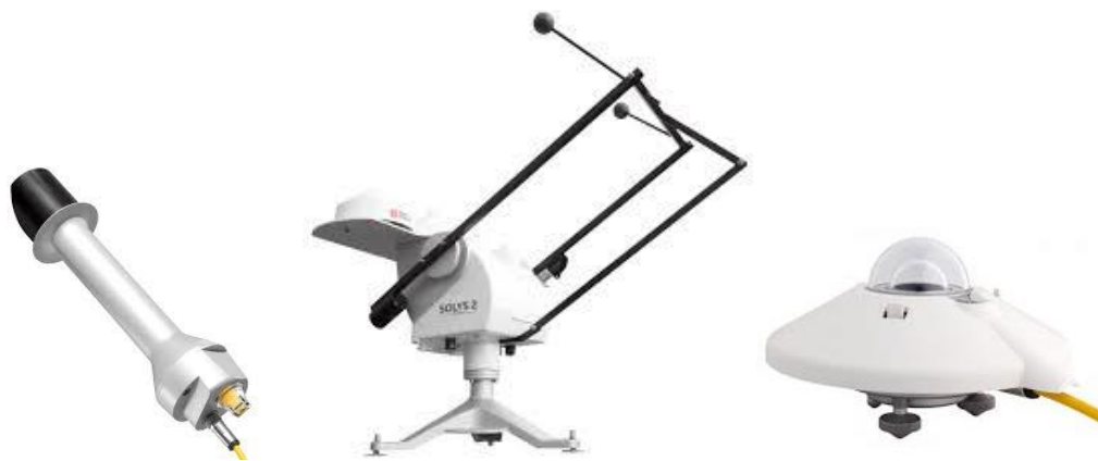
Figure 19 - Components of the weather station: (a) pyroheliometer, (b) solar tracker, (c) pyranometer
