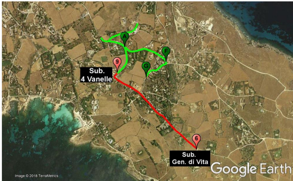
Fig. 63. Portion of Favignana distribution network under test: the MV line connecting the two secondary substations "4 Vanelle" and "G. Di Vita" is highlighted in red; the LV line departing from substation "4 Vanelle" is in green.
