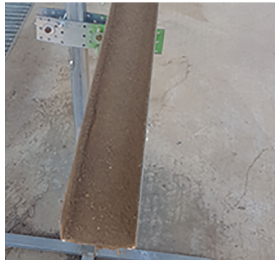
FIGURE 1 View of the flume covered by glued sieved soil
