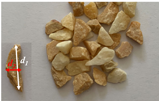
FIGURE 4 View of the measured largest ( d_1 ) and intermediate ( d_2 ) diameter of the gravel element
