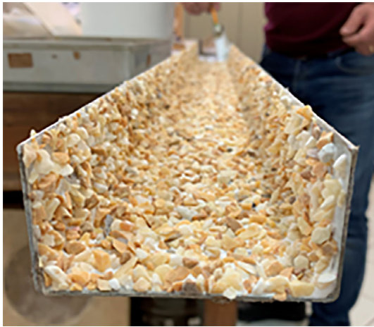
FIGURE 3 View of the flume covered by glued gravel
