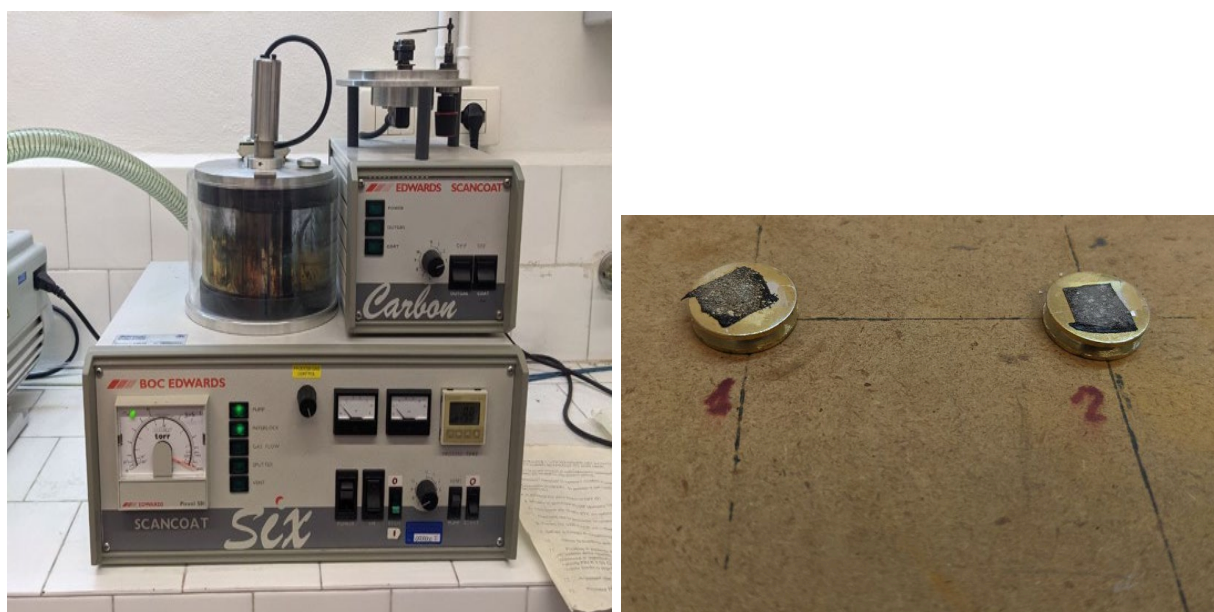
Figura 108 A sx: sputter coater 7 ; a dx: stubs pre-lavaggio
