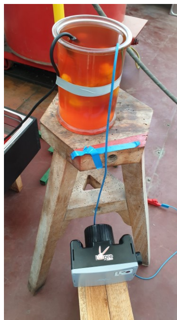
Figure 4.3. Arrangement of the cell immersed in mineral oil kept at room temperature
