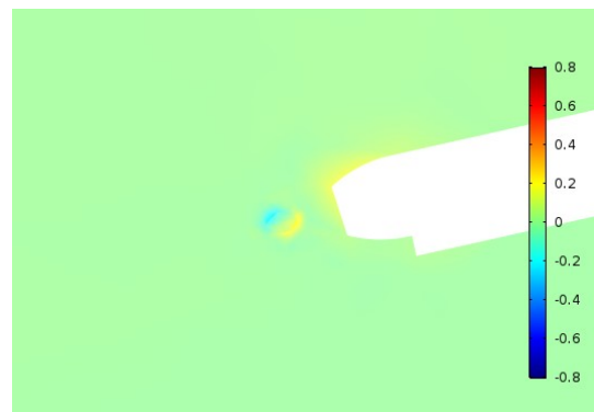
Figure 1.34. Space charge distribution before the inception of the first PD, after 1.4 ms from the beginning of the TOV (units in \text{C/m}^3 )
