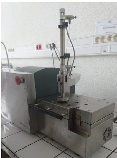
Figura A7: Mini Estrusore HAAKE MINILAB
