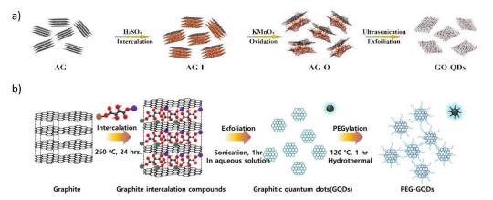
Figure 3. Schematics for the synthesis of graphene quantum dots. (a) Chemical intercalation and oxidation of aphanitic graphite. Figure adapted from Reference [111]. Copyright 2020, MDPI AG.
