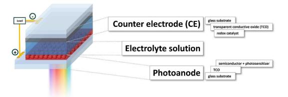
**Figure 6.** Schematic representation of DSSC's architecture. Due to their features, GQDs can be potentially applied as constituents of all three of the main components of DSSCs to further boost their performance.
