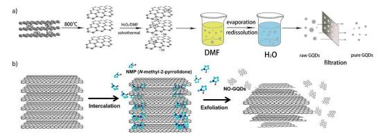
**Figure 4.** Schematic representation of GQDs prepared by solvothermal method according to (**a**) Tian et al. (Figure adapted from Reference [119]. Copyright 2016, Elsevier B.V.) and (**b**) Kang et al. (Figure adapted from Reference [121]. Copyright 2019, Elsevier B.V.).
