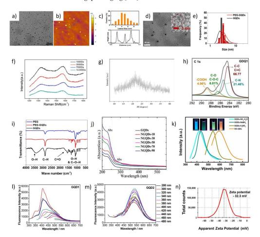
**Figure 5.** Methods for GQD characterization: (**a**) TEM picture, (**b**) AFM picture, (**c**) size and height distribution. Figures adapted from Reference [111]. Copyright 2020, MDPI AG. (**d**) HR-TEM picture of GQDs. Figure adapted from Reference [154].
