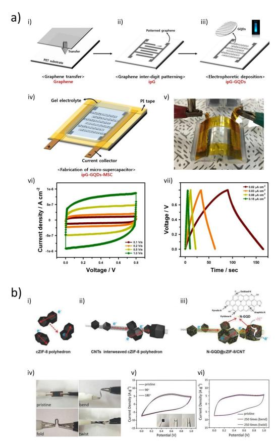
**Figure 8.** Supercapacitor architectures integrating GQD-based electrodes. (a) Schematic illustration for fabrication of an ipG-GQD-MSC: (i) Monolayer graphene prepared by CVD is transferred onto a PET substrate; (ii) the graphene is patterned
